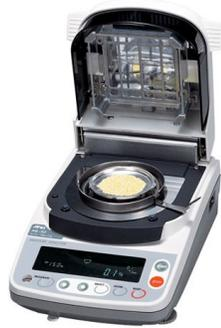
A moisture analyser with a 0.001g resolution and an accuracy of +/- 2 divisions will have a maximum accuracy (in a perfect test conditions) of +/- 0.02% and in the real world the accuracy may slip to +/- 0.04% and this is not be good enough if you need to know if the moisture content is below 0.1% when the balance is displaying 0.08%.
